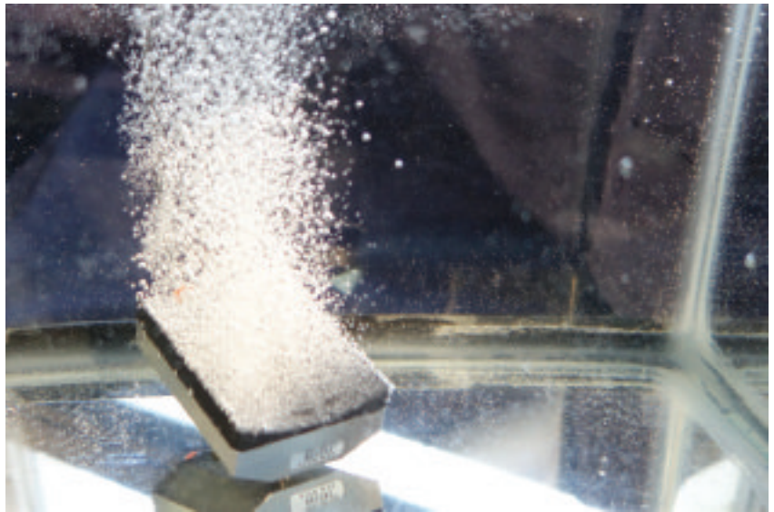
■ Figure 1. Air Pressure bleeds uniformly out of the entire face area of submerged externally pressurized porous tilt pad journal bearing.
